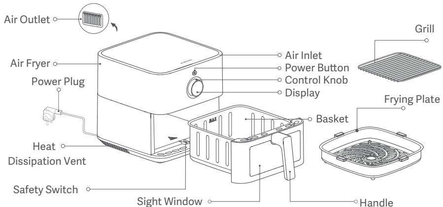
Notes: 1. The silicone rubber on the frying plate is made of high temperature resistant food-grade materials to prevent the edges of the frying plate from scratching the coating of the basket and to improve the stability of the frying plate. Do not remove the silicone rubber from the frying plate.
